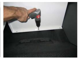
Pre-drill holes using 3/16" drill bit and attach using <sup>1</sup>/4"x 1" Lag bolts
